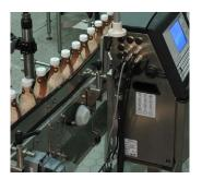
Series large character continuous ink jet printers from Videojet. The cases are coded with identification information and bar codes in much the same way the labels are used on the shrink-wrapped trays. The combination of human-readable information and bar codes enables customers to determine what is packaged in a case and scan the information into warehouse management systems to track shipping and receiving activities.
